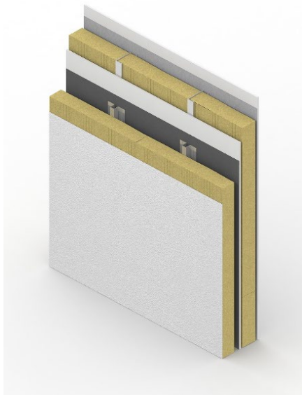
Diagram 4 - Typical build-up with LGSF and render system finishes
